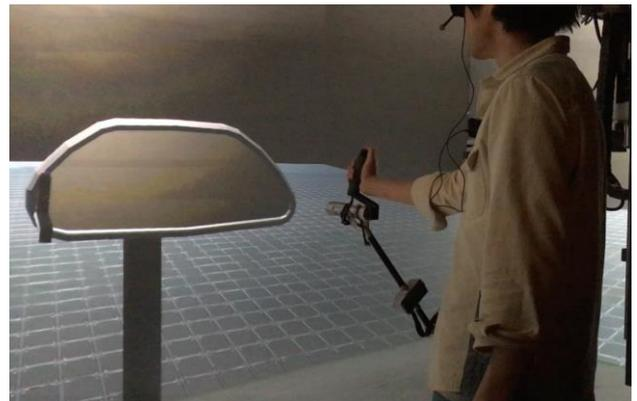
User modifying a CAD part in the EVE system using "Haption Scale One" haptic device.
